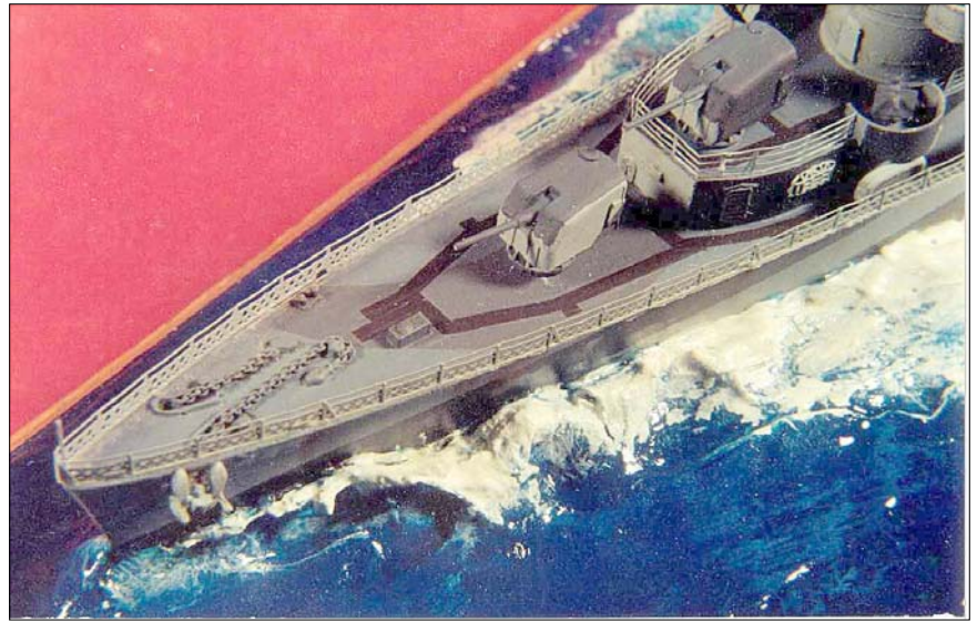
The Flagship Models photo-etch rails on the bow of this 1/350 Tamiya Fletcher is a good example of the advantages of raised etched relief on the parts. Note how the stanchions and bracing are thicker than the rails. Without computers, this feature would be almost impossible to create by hand.
